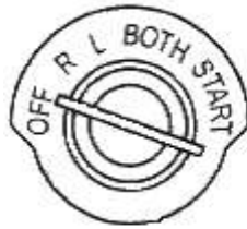
Fig. 10-7: Ignition selection switch
